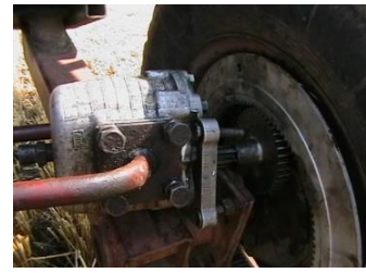
Fig. 2. General view of the hydraulic drive on the field support wheel of the harvester
