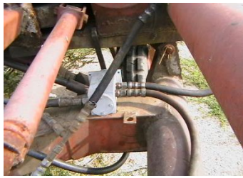
Fig. 1. Connection of the hydraulic distributor to the control system of the hydraulic motor on the field support wheel
